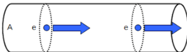
Figure 7.11: Flow of charge carriers
