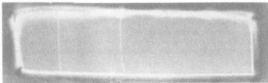
Fig. 3.57. Micrograph of the opening of the rectangular capillary with a macrostep photographed at different times to measure its rate of advance. (V. Bostanov, G. Staikov and D. K. Roe, J. Electrochem. Soc. 122, 1301 (1975). By permission of Electrochemical Society Inc. and courtesy of V. Bostanov.)
