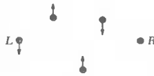
Figure 9 Short phonon mean free path in a disordered structure. A short wavelength phonon that displaces atom L, as shown, will displace atom R by a much smaller distance, because of the phase cancellation of the upper and lower paths from L to R. The displacement of R is \uparrow + \downarrow \sim 0 , so that the wave incident from L is reflected at R.
