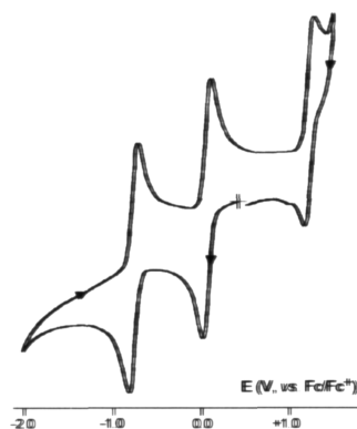
Figure 5. Cyclic voltammogram recorded in \text{CH}_2\text{Cl}_2 solution of [\text{Ni}(\text{dphedt})_2] . Scan rate 0.2 \text{ V s}^{-1} .
