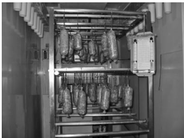
Figure 18.4. Sausage stuffed into a collagen casing, 80-mm diameter, and clipped on both extremes.
