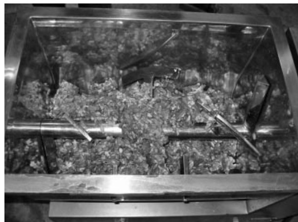
Figure 18.3. Detail of the batter after mixing in a vacuum mixer massager.
