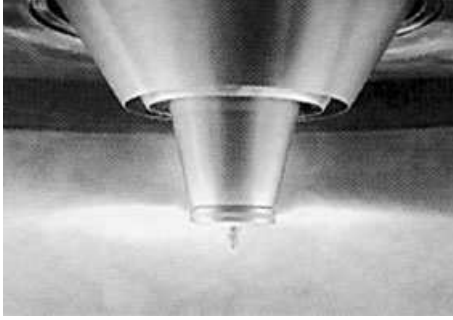
Fig. 3.12 Centrifugal atomiser; by courtesy of Niro.
