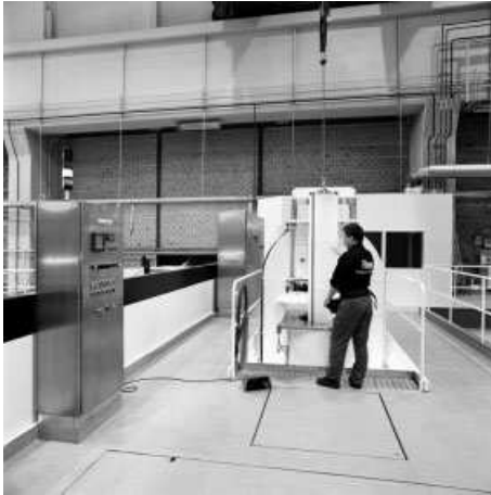
Fig. 6.5 Illustration of a 'batch' HPP system; courtesy Avure Technologies AB.
