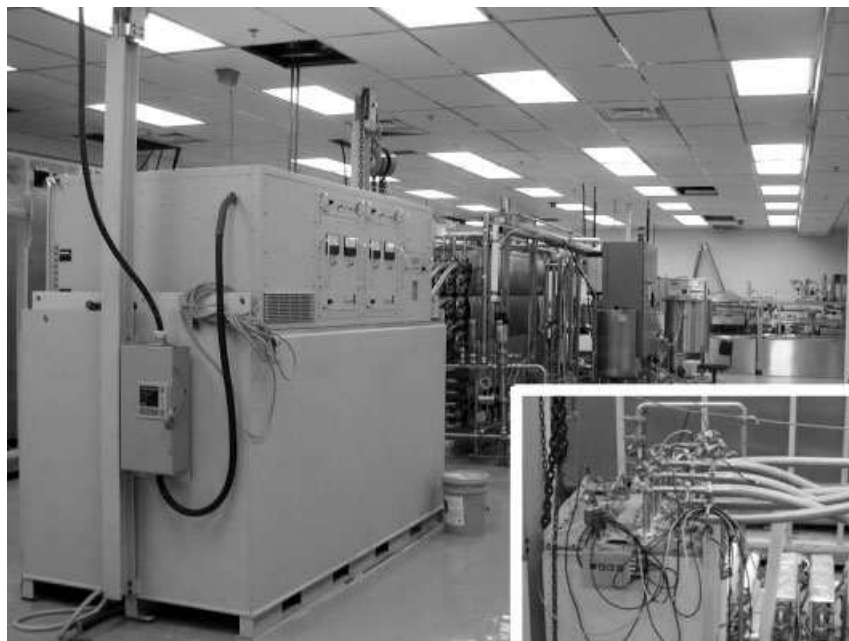
Fig. 7.3 Continuous-flow PEF processing: 'OSU-6' at the Ohio State University (picture courtesy of Prof. Howard Zhang, The Ohio State University).
