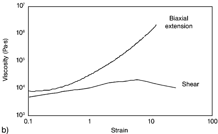
Fig. 8.10 Effect of polymer chain branching on shear and extensional viscosities of (a) branched low-density polyethylene at 125 °C and (b) dough.
