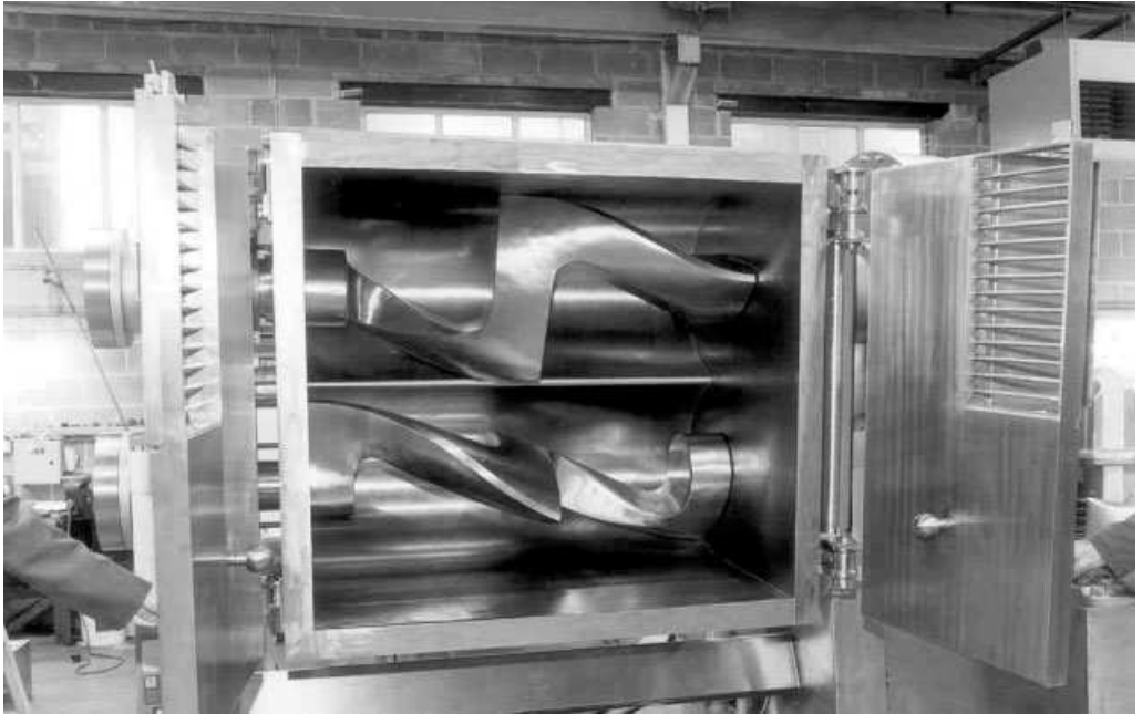
Fig. 15.7 Z-blade ( \Sigma -blade) mixer; by courtesy of Winkworth Machinery Ltd.
