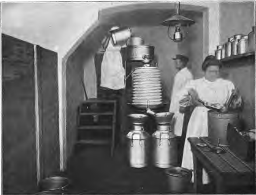
FIG. 55.—Cooling and Straining of Milk at Fauerholm. In the foreground Ice is being put into the bottom of Busck's Milk Pail.
