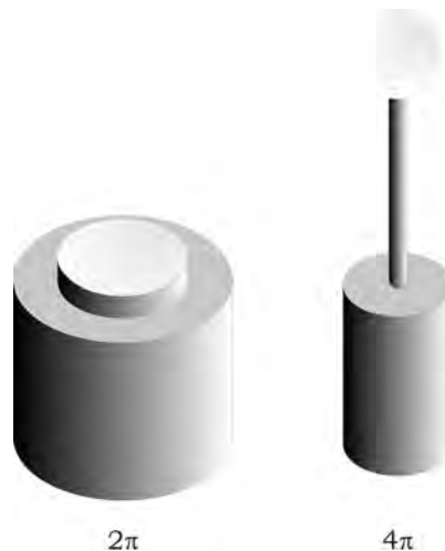
FIGURE 5.14 Examples of PAR detectors equipped with a planar 2\pi collector or with a spherical 4\pi collector.
