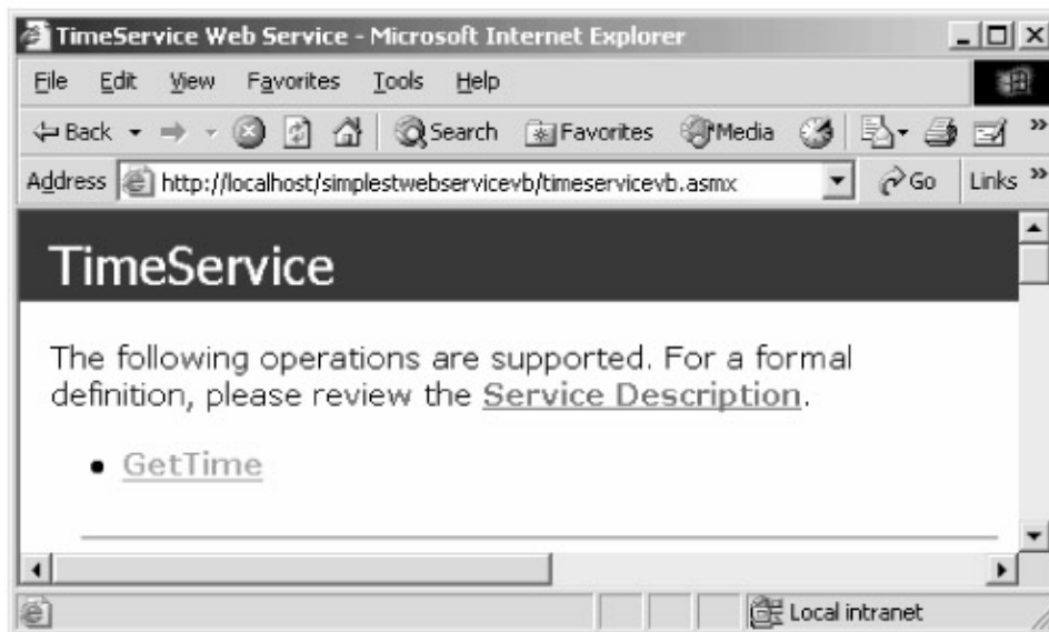
Figure 4–5: Default screen generated by ASP.NET when you request the XML Web service base page.
