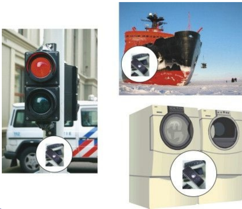
Figure 1.2 Embedded systems are microprocessor-equipped systems and devices that interact with the physical world. Examples include traffic lights, a ship's rudder controllers, and washing machine controllers.
