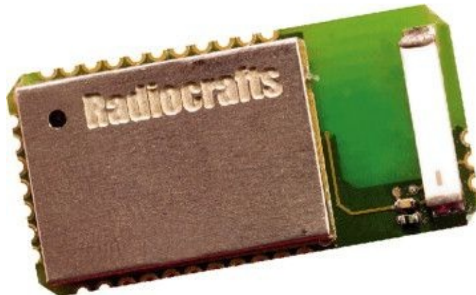
Figure 11.3 Texas Instruments CC2430 single-chip radio transceiver with integrated 8051 microcontroller and onboard antenna manufactured by Radiocrafts. The size of the board is 1.2 \times 1.0 \text{ cm}^2 .
