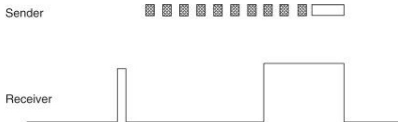
Figure 11.21 To transmit a packet with LPL, the sender first sends a series of strobe packets to wake the receiver up.
