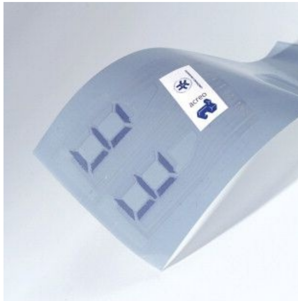
Figure 11.7 Printed electronics allow circuits and simple displays to be printed using a regular ink-jet printer.
