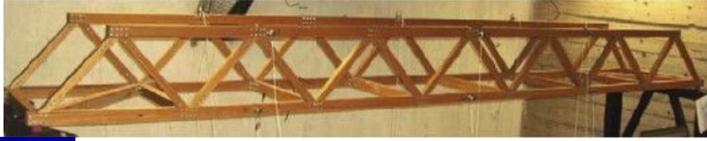
Figure 25.1 Experimental bridge used for SHM studies.
