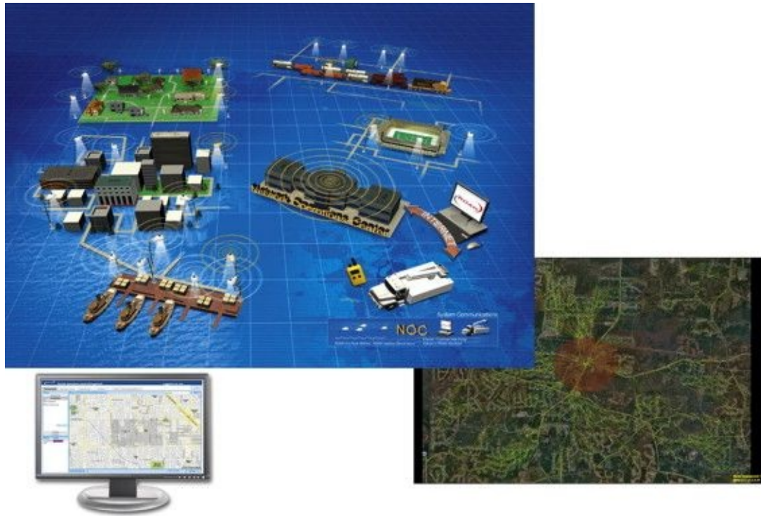
Figure 22.3 ROAM lighting management networks.
