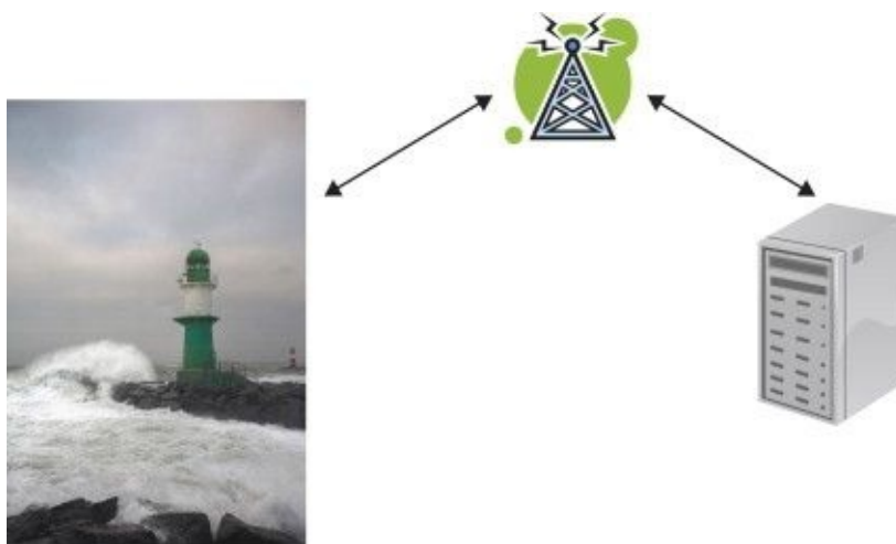
Figure 1.4 Telemetry allows reading measurements from remote systems such as weather stations. Data are typically transported using mobile telephony systems.
