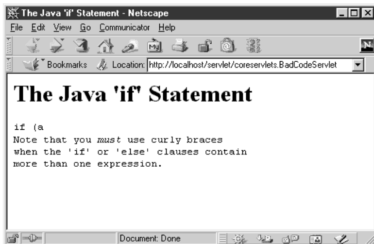
Figure 3-9 Result of BadCodeServlet : much of the code fragment is lost, and the text following the code fragment is incorrectly displayed in a monospaced font.
