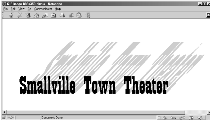
Figure 7-7 Using the GIF-generation servlet to build the title image for a site describing a local theater company.
