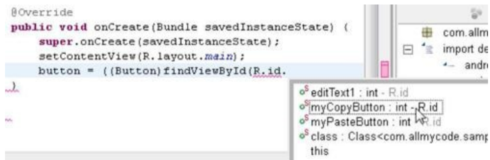
Figure 1-20: The Eclipse editor is aware of the names you create in your Java code.
