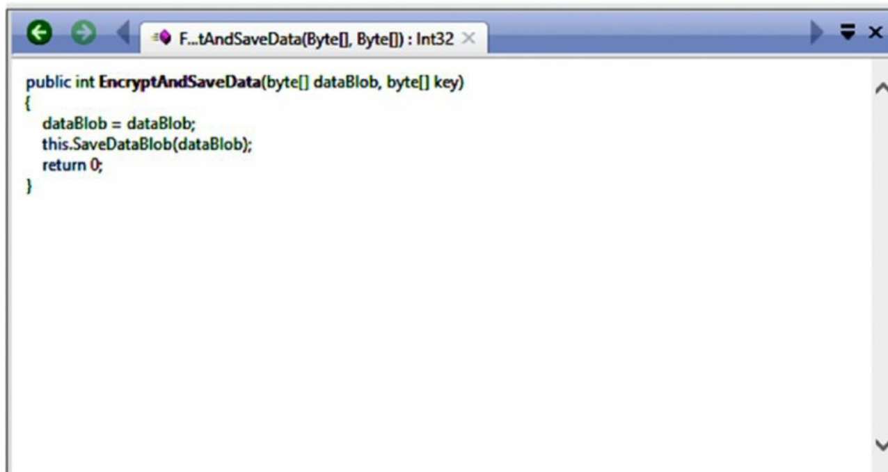
Figure 11.19 New disassembly for SaveAndEncryptData() after patching the method Success! The patched assembly now clearly bypasses the undesired crypto code path.
