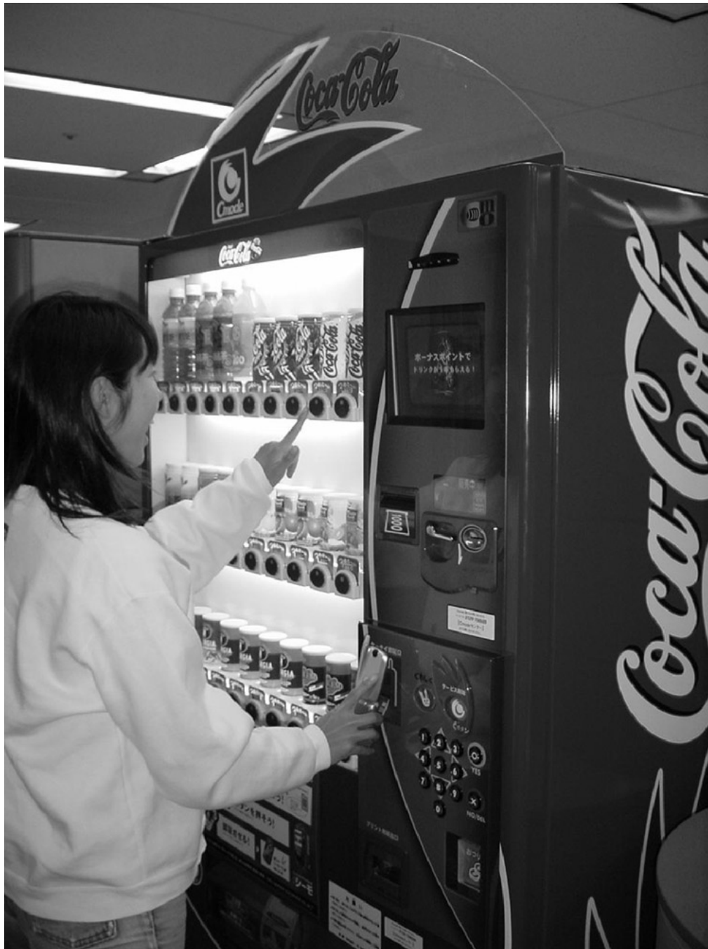
Figure 6: Coca-Cola's C-Mode. Next generation vending machine with barcode reader and video screen, which, when linked with i-mode, becomes not only a drink dispenser but also a multimedia terminal, capable of ticketing, and more
