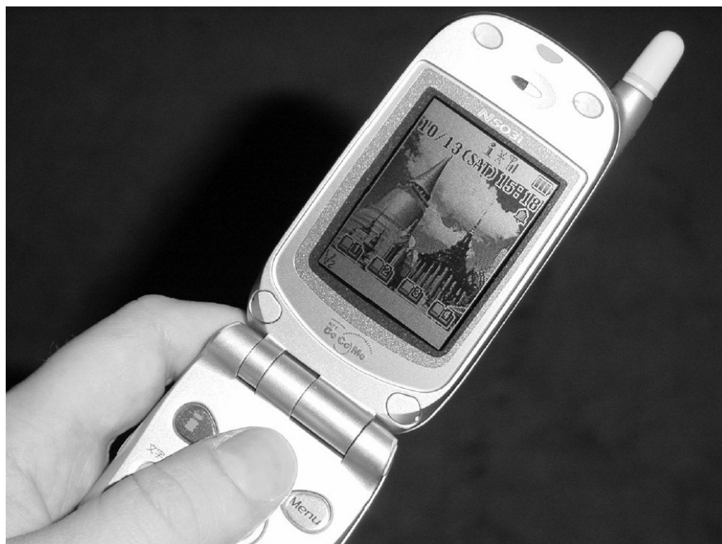
Figure 2: 503i Series Handset (NEC). 503i series handsets all contain Sun Micro-systems Java technology and full-colour displays. These features, in addition to the 16-voice ringing tones, offer the user an advanced handset for either business or pleasure.
